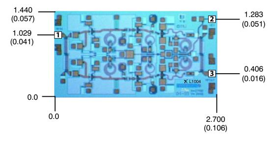
Units: millimeters (inches) Bond pad dimensions are shown to center of bond pad. Thickness: 0.110 +/- 0.010 (0.0043 +/- 0.0004), Backside is ground, Bond Pad/Backside Metallization: Gold All Bond Pads are 0.100 x 0.100 (0.004 x 0.004). Bond pad centers are approximately 0.109 (0.004) from the edge of the chip. Dicing tolerance: +/- 0.005 (+/- 0.0002). Approximate weight: 2.411 mg.
